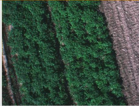
Example image of the sample field taken by the drone, color image generated by fusing the RGB-like spectral images.
